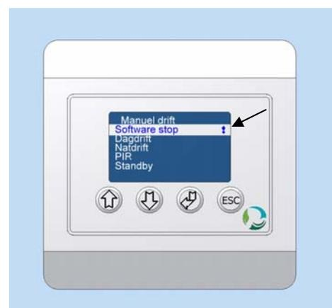
The software stop function has now been activated and the display shows an exclamation mark (!).
