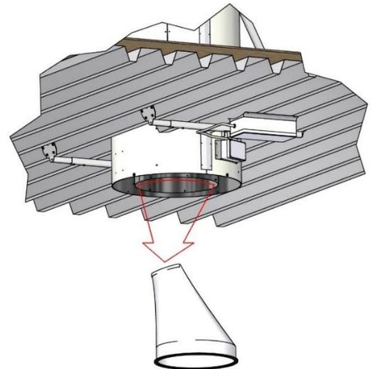
The inner tube of the bottom extension unit is placed in the inner tube of the unit and fixed in place using 7 Ø5,5 self-drilling screws.
