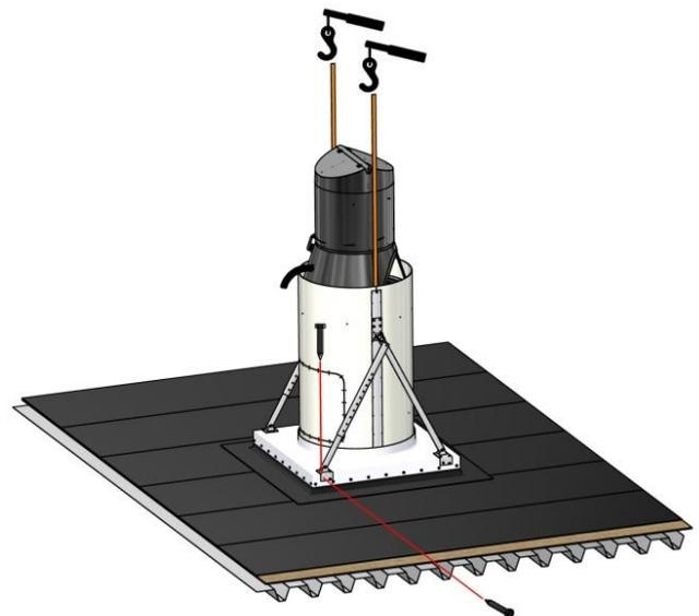
Bolt and nut is installed through the holes of the fork shaped brackets so they lock the mounting studs in place as shown in the illustration.
