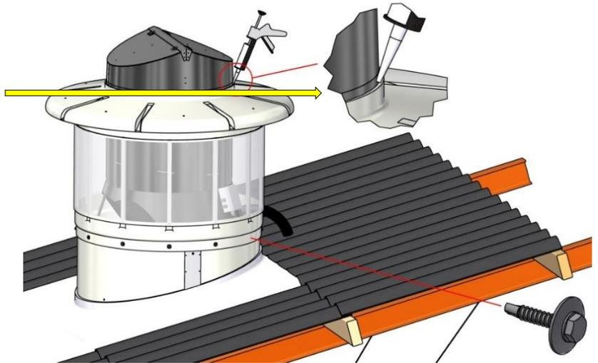
The top cone is installed by placing it on top of the filter holder.
