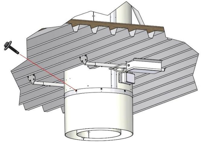
The inlet ring is installed by pushing it over the 2 tubes in the bottom extension unit. The inlet ring is fastened from the inside tube with the 7 included chipboard screws and from the outside with the 4 included self-drilling gasket screws.
