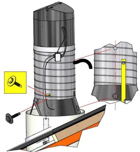
The wiring is installed according to the wiring diagrams in **4.0 Electrical wiring diagrams**
