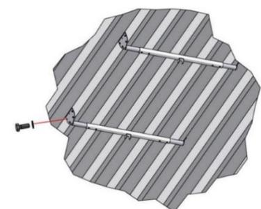
The two trapezoidal brackets are fixed to the trapezoidal profiles using the included 16 M8 bolts and washers.
