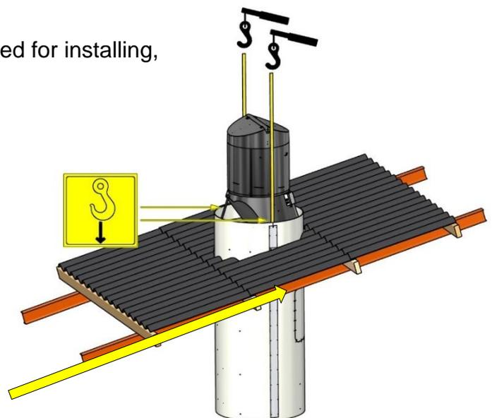
The unit is hoisted or lowered in place so that the mounting studs fall into place in the fork shaped brackets of the standard mounting brackets. It is checked that the unit is plumb.
