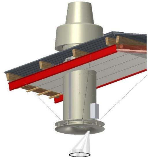
The filter is kept in place by the rubber profile situated around the edge of the filter's collar. The rubber seal must be placed so the circular part is facing outwards. Otherwise air leakage will occur and there will be a fall hazard of the filter
