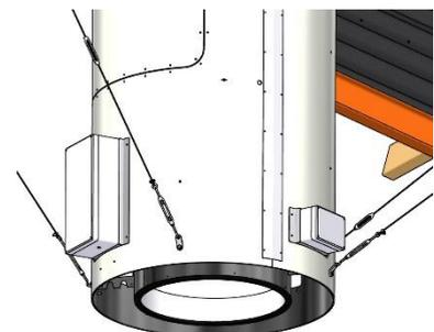
In the center of the soft cover a hole is cut. It is recommended to use the template from **2.4 Template** as reference. It must be taken into consideration when cutting the hole that the soft cover should be placed under either overlying roof plate(s) or the ridge of the roof with an overlap of minimum 100 mm.
