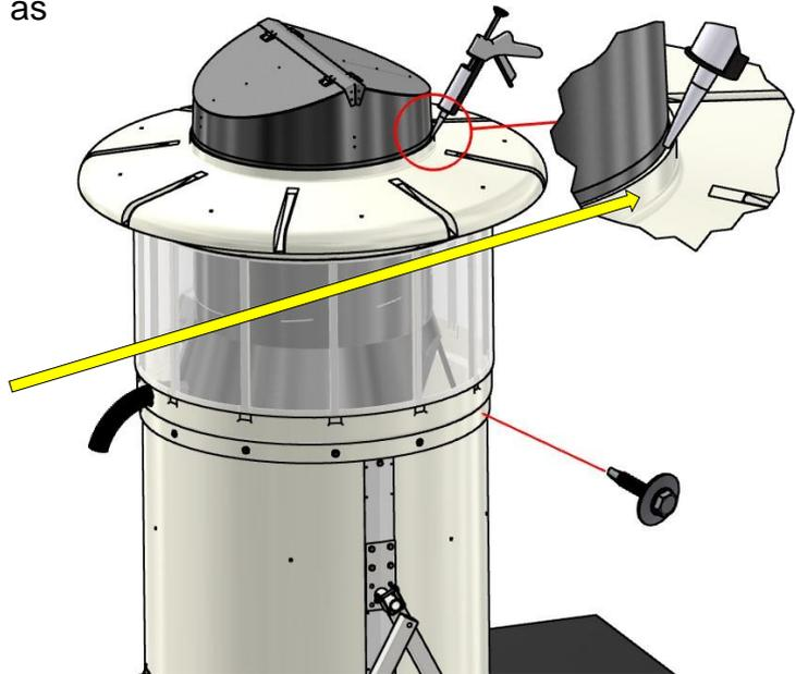
The top cone is installed by placing it on top of the filter holder.
