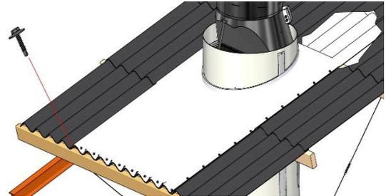
The overlying roof plate(s) the ridge of the roof is lifted to put the soft cover beneath it. The soft cover is fastened with the included Ø5,5 mm self-drilling screws, up to 50 screws, with a distance between them of approximately 200 mm or as required to ensure proper seal with the roof.
