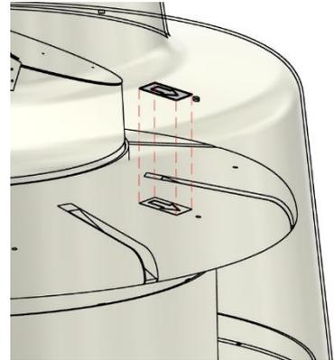
The top cone is attached to the filter holder with the included 4 M8x20 mm bolts and washers.
