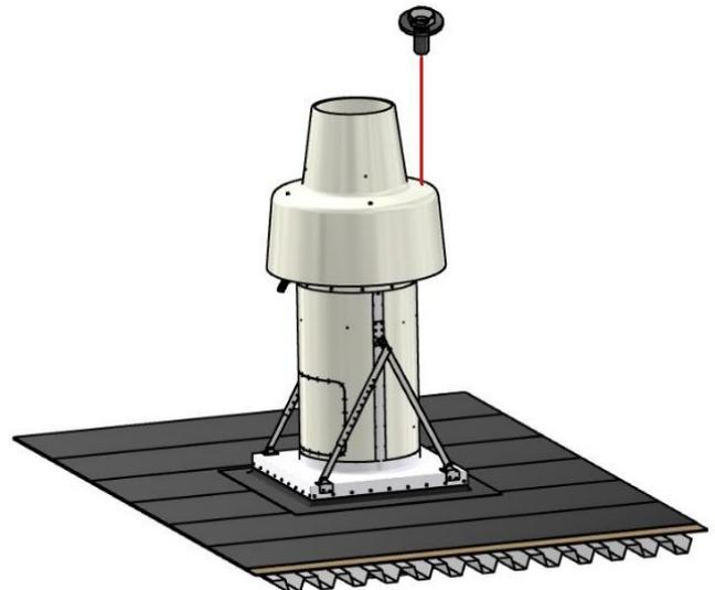
The inlet ring is installed by pushing it over the 2 tubes in the unit. The inlet ring is fastened from the inside tube with the 7 included chipboard screws and from the outside with the 4 included self-drilling gasket screws.
