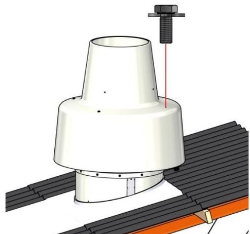
The inlet ring is installed by pushing it over the 2 tubes in the unit. The inlet ring is fastened from the inside tube with the 7 included chipboard screws and from the outside with the 4 included self-drilling gasket screws.
