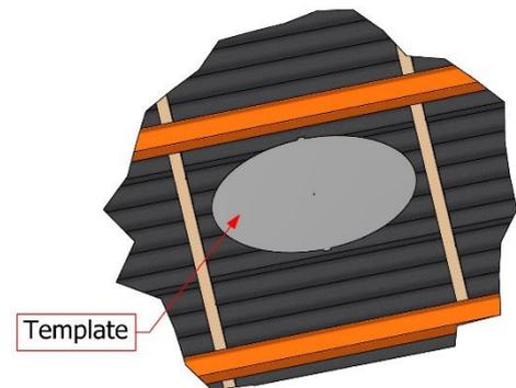
A hole is then drilled or cut vertically through the roof.
