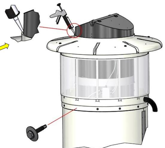
The top cone is installed by placing it on top of the filter holder.
