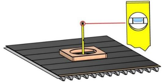
Asphalt roofing is applied so that it aligns with the top of the wooden frame and creates a sealed overlap on the roofing of the roof.
