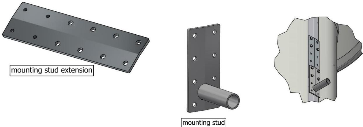
The mounting stud extensions are attached to the TX3100A unit using the long M8 bolts and washers with which the mounting studs were attached by default. The mounting studs are attached to the mounting stud extensions using the short M8 bolts and washers that comes with the mounting stud extensions.
