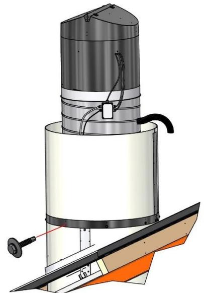
The filter holder is attached with the 12 included self-drilling screws. A silicone grout joint is laid all around the top against the unit as shown in the illustration.
