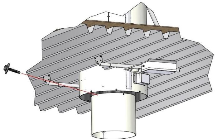
The outer tube of the bottom extension unit is placed over the outer tube of the unit and fixed in place using 10 Ø5,5 mm self-drilling screws.
