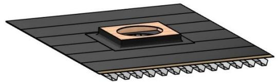
The soft cover is cut with the measurements of 1400x1400 mm and a hole for the unit is cut in the center of the soft cover.
