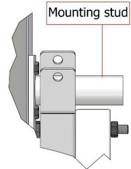
The unit is hoisted or lowered in place so that the mounting studs fall into place in the fork shaped brackets of the adjustable mounting brackets. It is checked that the unit is plumb. The adjustable mounting brackets is fixed to the wooden frame through the soft cover using the 16 included wood screws.
