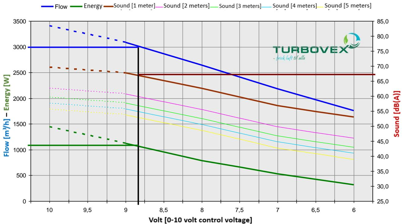
The airflow indicates the balanced air exchange in relation to the control voltage. (0-10 volt) and is shown in m<sup>3</sup>/h. The unit can be adjusted manually to suit your required air exchange.
