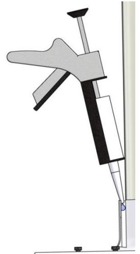
A joint of silicone rubber grout is laid where the softcover meets the unit. The softcover is pressed against the unit by hand to ensure seal between the soft cover and unit.
