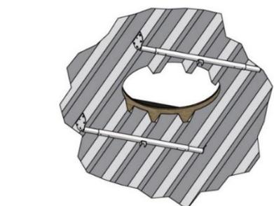
Using the center mark and the 2 trapezoidal brackets as reference (optionally using the template in **2.4 Template**) a Ø890 hole is cut through the roof.
