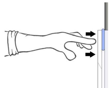
The filter holder is attached with the 12 included self-drilling screws. A silicone grout joint is laid all around the top against the unit as shown in the illustration.
