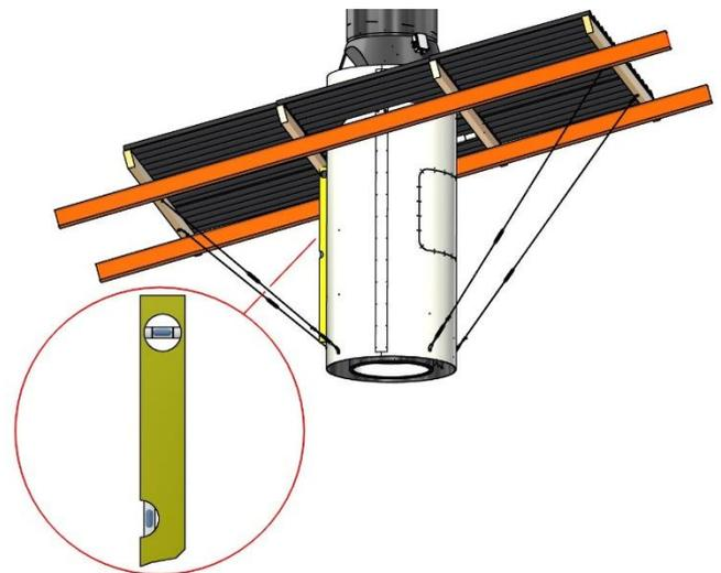
With the unit and wires installed, fixed and adjusted the 2 electrical boxes can be re-attached to the unit.
