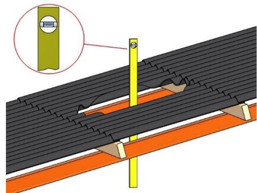
According to the placement of the unit it is measured where the two standard mounting brackets should be installed with a distance between them of 1000 mm, so that the unit is placed equally distanced from both.
