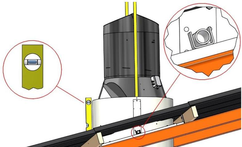
If the 4 wire brackets were temporarily removed for installing the unit, they are now re-attached to the unit.
