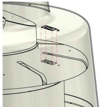
The top cone is attached to the filter holder with the included 4 M8x20 mm bolts and washers.
